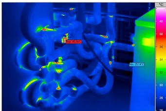
In the evaluation phase of the project, system and assembly-related insulation weaknesses will be identified and optimised using prefabricated components.
